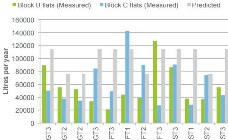
All the flats in the development were designed to comply with level 3 of the CSH, predicting the daily use of potable water to be 105 litres per person
