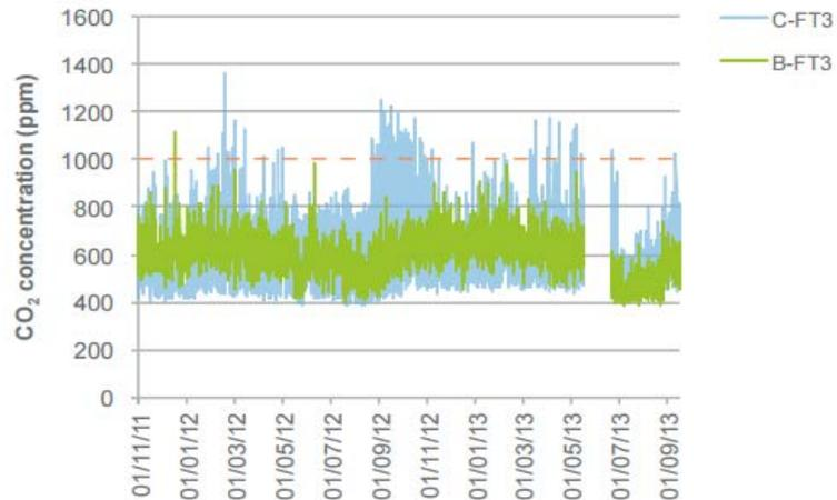
Measured CO<sub>2</sub> concentration levels were below the 1000ppm limit for most of the project's duration.
