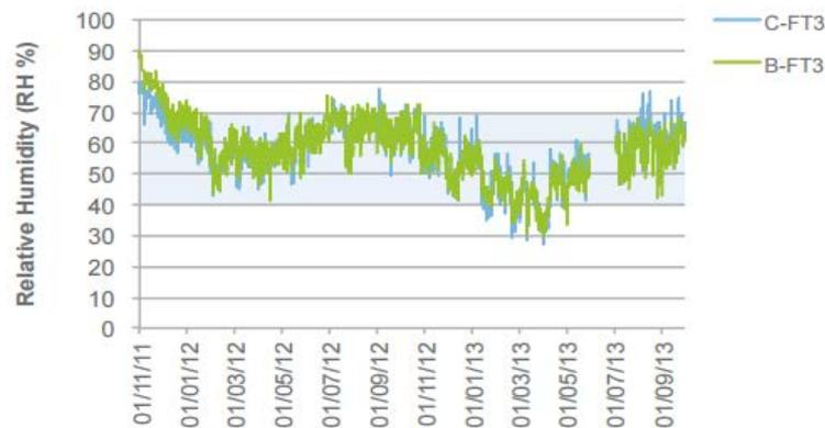
The humidity levels in both sub-metered flats were within the acceptable range for most of the project's duration.
