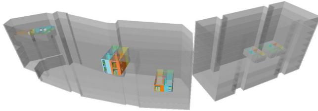
Dynamic thermal simulation models are powerful software tools, which model the energy interactions and internal environmental conditions in a building on an hour-by-hour basis.
