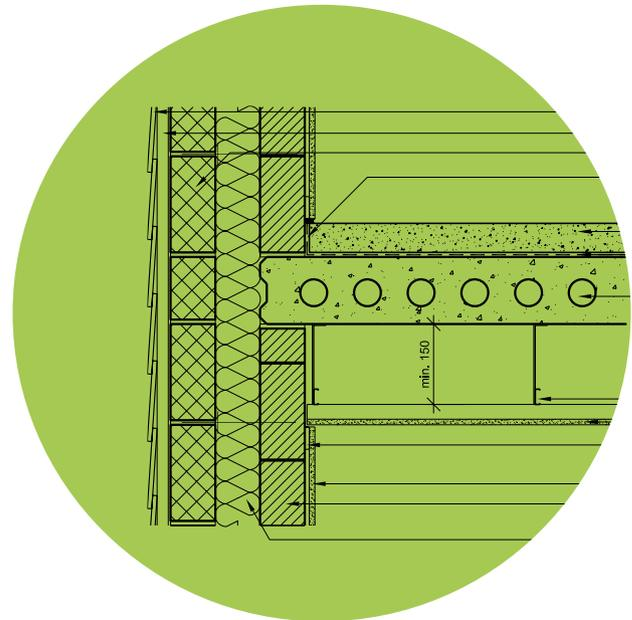
*Floor detail (Robust Detail E-FC-4)*
