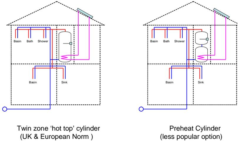
Heat pumps generally tend to be most efficient at producing temperatures of up to around 45°C. Whilst some will go higher this is inevitably at the expense of efficiency. In all cases an additional back up heat source is required for periods when Thermal Solar is not sufficient and/or to boost the delivery temperature.
